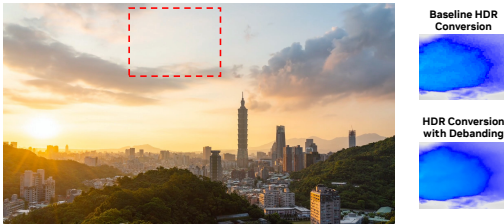
Figure 4. Visualization of changes in luminance between a baseline HDR conversion and one with debanding as implemented in RTX HDR. Input video by Timo Volz from Pixabay.
